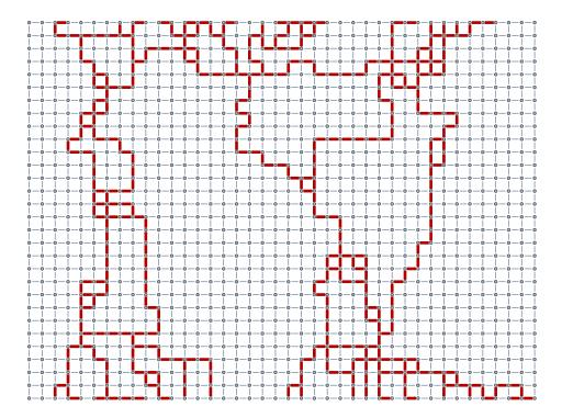
This numerical experiment confirms that the percolation threshold is between 0.3 and 0.55. Indeed, for the bond percolation on the square lattice  $\mathbb{Z}^2$  we know that  $\phi_c = 1/2$ . The proof of this fact is non-elementary<sup>1</sup>.
